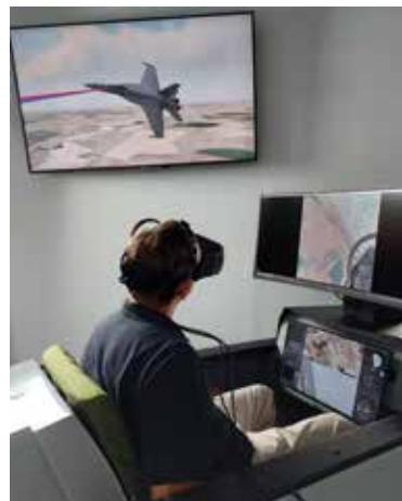
Left: VRSG view on the wall-mounted monitor shows the ability to track the pilot's head position and orientation, track the gaze vector using the Varjo XR-3's pupil tracking functionality, and then visualize the gaze of each eye independently as a color-coded 3D cone. Right: Adjustable (patent pending) control stick for side- or center-stick positioning.
