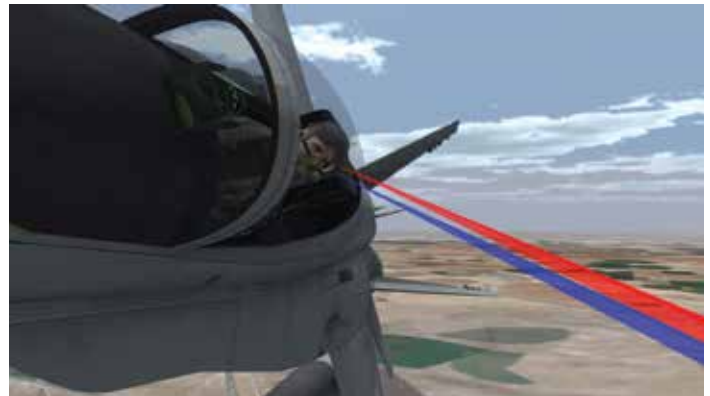
VRSG real-time scene visualizing the gaze of the wearer of a Varjo XR-3 mixed-reality headset through the collection of eye-tracking data.
