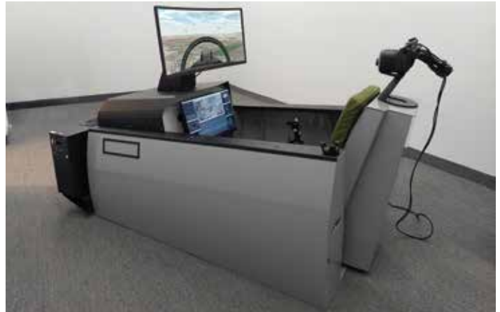
Part Task Mission Trainer (PTMT) with Varjo XR-3 mixed-reality system.
