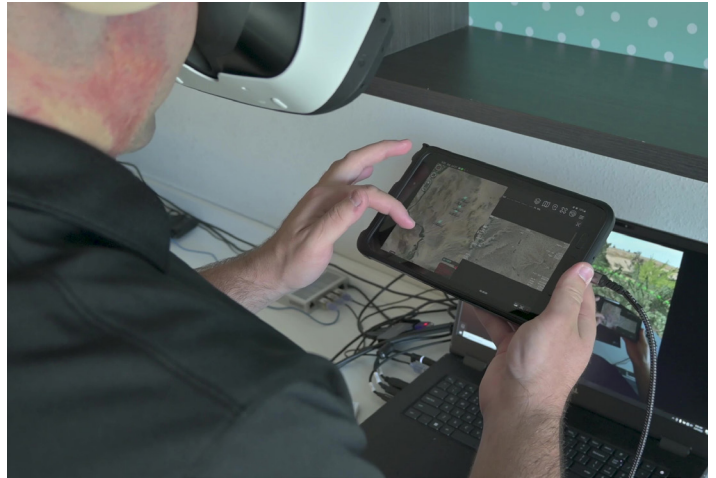
The JTAC Backpack provides an ultra-portable mixed-reality training device that supports real-world video pass-thru. The observer can interact with real end user devices and stay immersed in the virtual environment.
