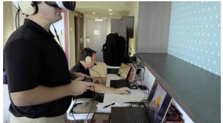
JTAC student using simulated HUDs in the head-mounted display for the LTD and LRF to support a terminal attack. Correlated views of the impact can be seen in the HMD view and the sensor pod view.
